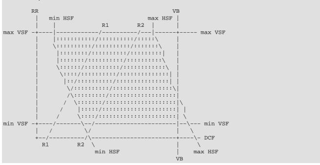
This is a generic monitor mode diagram. The x axis of the diagram shows the clock rate (DCF), the y axis represents the refresh rate (RR). The filled region of the diagram describes the monitor's capabilities: every point within this region is a possible video mode.
